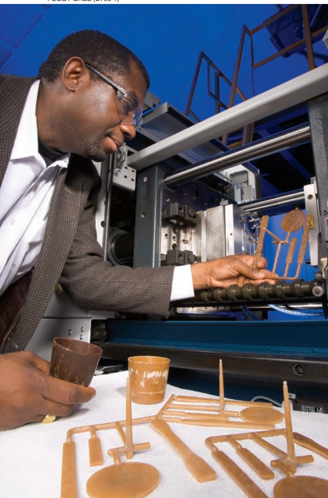
Food technologist Charles Onwulata inspects molded dairy bioplastic made from surplus whey proteins.
