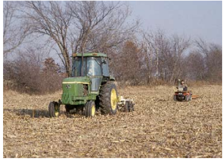
Two commercial soil electrical conductivity (EC) sensors were used to map soil variability and develop productivity zones. One is mounted on the back of the tractor and uses disk coulters contacting the soil to measure EC at two depths. The other, attached to the small vehicle behind the tractor, does not require soil contact but measures EC at only one depth.
