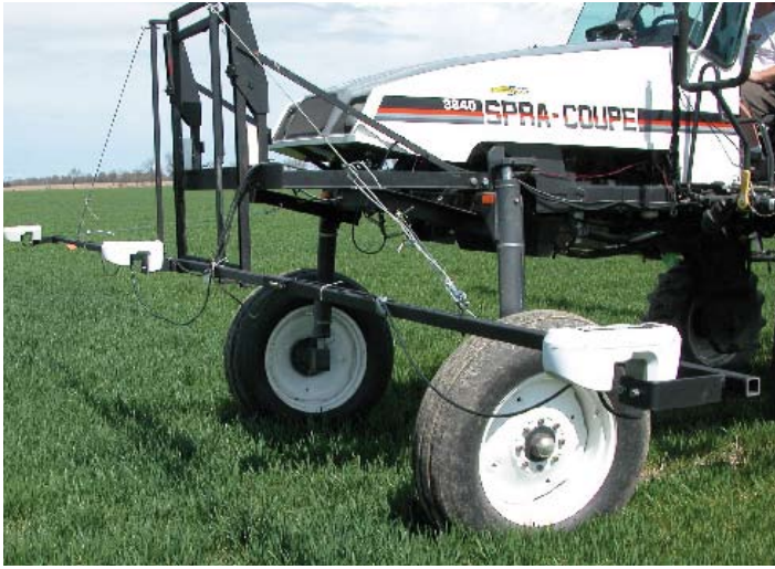
Light reflectance sensors mounted on the front of an applicator are used to measure nitrogen deficiency so that nitrogen can be applied as needed (at a variable rate) when the applicator moves through the field.
