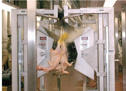
Broiler carcasses exiting an automated feather-picking machine in the pilot poultry processing facility at the Russell Research Center.
