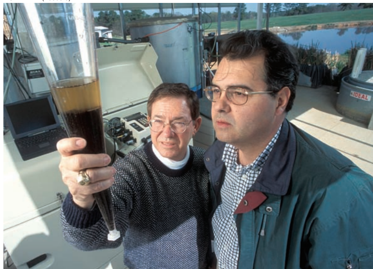
Soil scientists Patrick Hunt (left) and Matias Vanotti examine a sample of nitrifying pellets that can remove nitrogen in a hog-manure management system.
