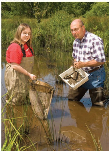
The small invertebrates being sampled by technician Lisa Williams and ecologist Charles Cooper are found in wetlands and ditches, where they are excellent indicators of the current quality of water and provide a way to measure improvements from in-field and edge-of-field conservation practices.
