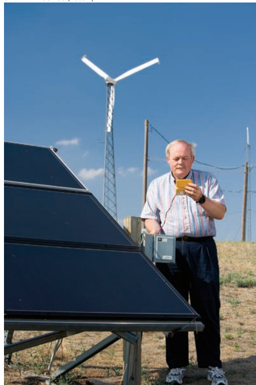
Agricultural engineer Brian Vick measures electrical current output from solar panels used for remote water pumping. The water is mainly used for livestock watering.
