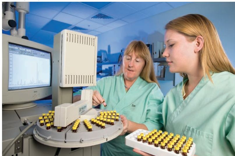
Technician Susan Crookall (left) and biological science aide Brittelle Bowers begin an analytical gas chromatography run.
