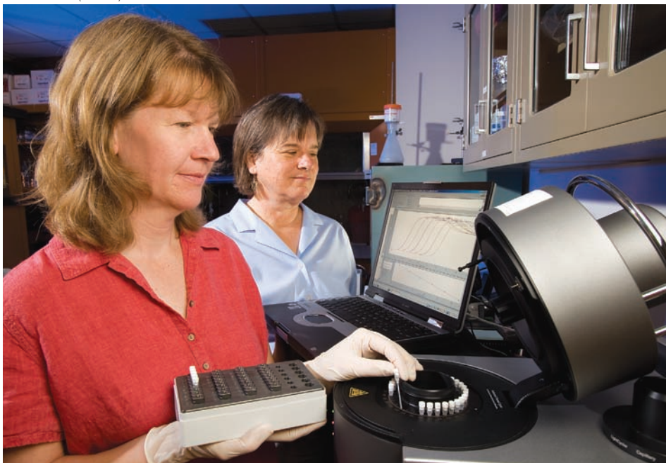
Technician Brenda Shaffer (left) and plant pathologist Joyce Loper load samples for quantitative PCR analysis, a procedure to evaluate gene expression by P. fluorescens Pf-5.
