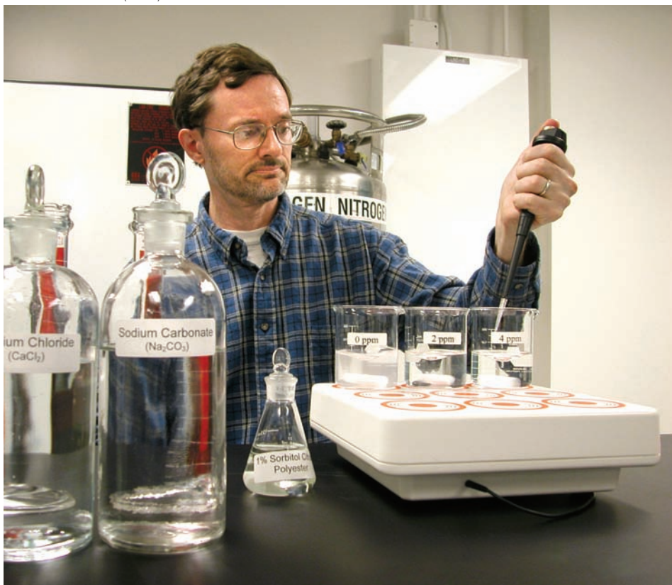
Chemist Randal Shogren performs a test to determine how much sorbitol citrate is needed to prevent scale, the crusty buildup of calcium carbonate from so-called hard water. Sorbitol citrate could be used as an inexpensive, environmentally friendly detergent additive.
