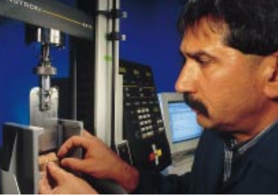
Physiologist Mohammad Koohmaraie uses an electronic testing machine to measure the tenderness of a sample sheared from a cooked steak.
