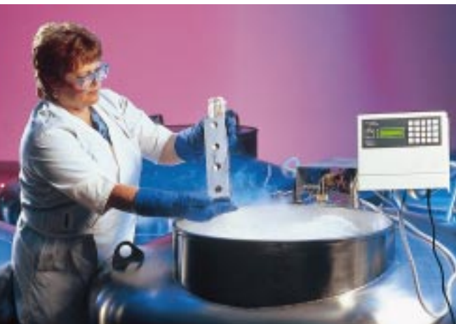
Technician Jolene Hansen examines seeds preserved in a vat of liquid nitrogen that can hold 5,000 containers of up to 2,000 seeds. The longevity of cryopreserved seeds is projected to be hundreds of years, but scientists periodically remove them to assess their viability and vigor.
