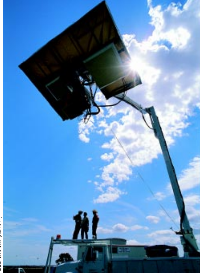
Microwave radiometers mounted on this boom truck can quickly measure soil moisture.
