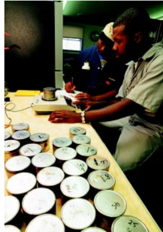
Alabama A&M University students Jimmy Moore (foreground) and Jacques Surrency weigh soil samples in preparation for moisture measurements.
