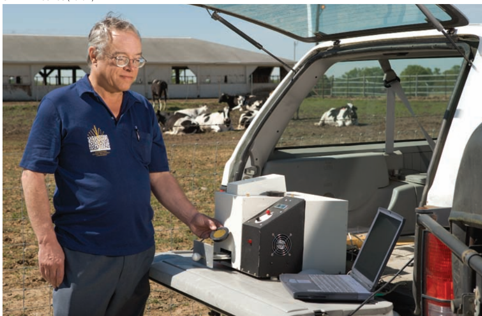
Chemist James Reeves analyzes manure for nitrogen in the field using a prototype near-infrared filter spectrometer.
