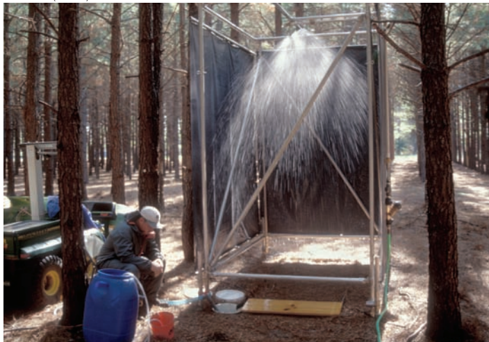
Using a rainfall simulator, technician Steve Haller collects runoff from a loblolly pine stand to determine the effects of pine straw harvesting on water, soil, and nutrient losses.
