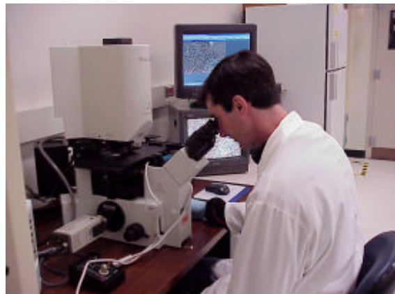
The laser capture microdissection instrument can be used to collect individual cells from tissues sections. Then the cells can be analyzed for genomic and proteomic alterations.
