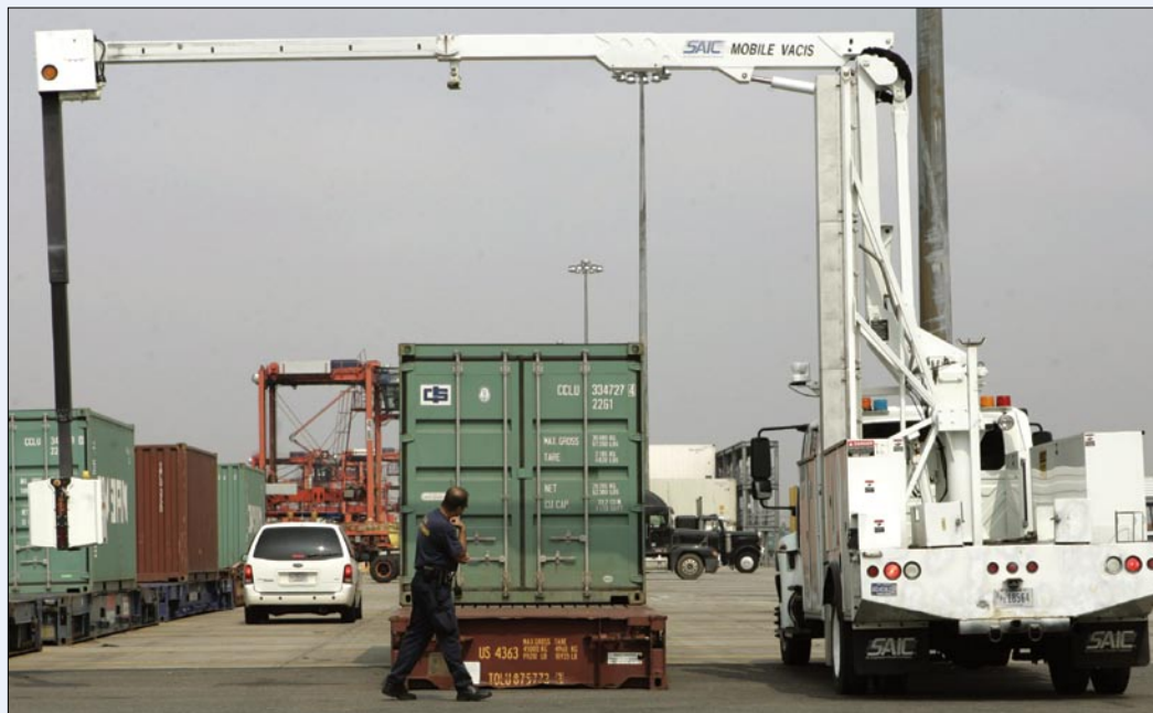
A mobile radiation detector screens cargo for dirty bombs or terrorist weapons at Port Newark in New Jersey, July 2006. AP/Wide World
