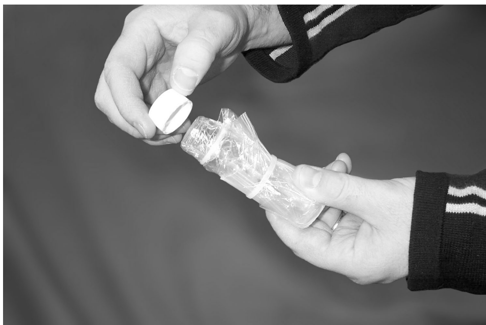
Figure 8. Screwing a septated cap onto a glass vial encased in the inner low-density polyethylene tubing.
