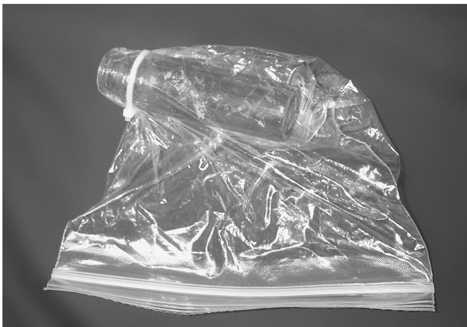
Figure 4. Glass vial positioned in sandwich bag so that a single layer of low-density polyethylene is tight across the opening and the self-locking nylon tie does not interfere with capping.
