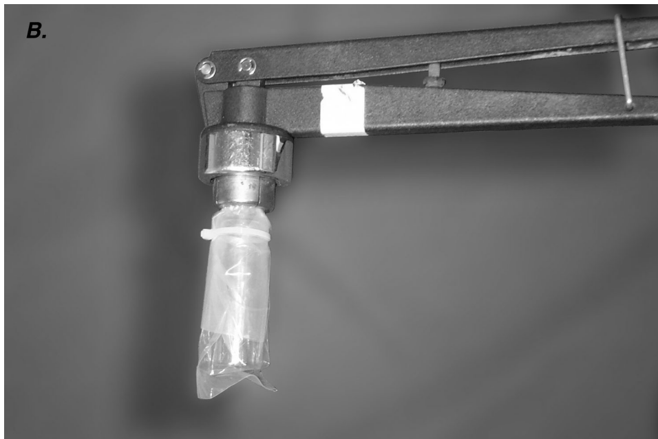
Figure 9. (A) Attaching and (B) crimping a septated cap onto a glass vial encased in the inner low-density polyethylene tubing.
