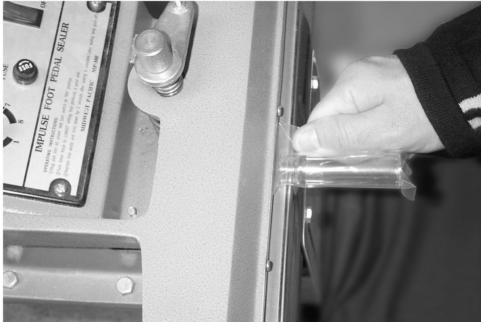
Figure 3. Heat sealing of glass vial in polyethylene tubing.
