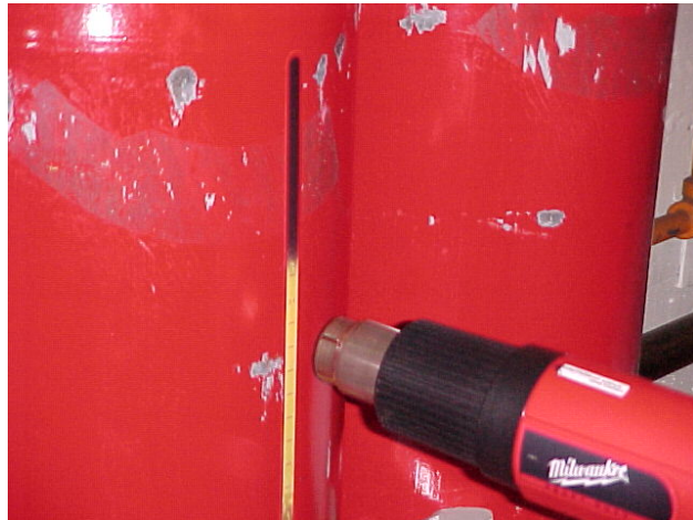
Figure 1. - Heating Liquid Level Strip
