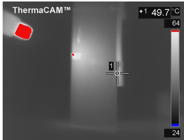
Figure 4. - Infrared picture of an ABC fire extinguisher while being heated with a heat gun. The white square areas on the extinguisher are black electrical tape.
