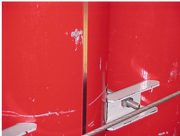
Figure 2. - Liquid Level Strip, showing level of CO 2
