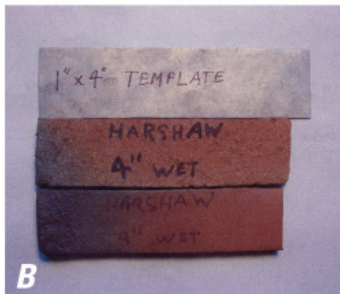
Figure 6. Test tiles of Harshaw clay. Clay samples were collected at locality shown in figures 4 and 5. R, pale-red variety of clay; Y, yellowish-gray variety of clay. “4 in. wet” notation printed on tiles refers to initial length (10.2 cm) when wet. A , Test tiles after drying but before firing. Tiles are about 9.2 cm long, demonstrating shrinkage of about 9 percent on drying. B , Test tiles after firing. Upper tile is 9.1 cm long, and lower tile is 8.9 cm long, demonstrating additional shrinkage of less than 1 percent on firing.
