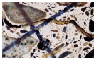
Figure 9. Polished sample of concrete, showing cracking induced by pressure from swelling alkali-silica gel. Crack extends through sand/cement matrix and passes by several coarse aggregate particles. Field of view, 20 by 55 mm.
