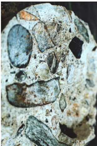
Figure 9. Polished sample of concrete, showing cracking induced by pressure from swelling alkali-silica gel. Crack extends through sand/cement matrix and passes by several coarse aggregate particles. Field of view, 20 by 55 mm.
