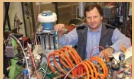
Anatoly Zelenski is pictured with the optically pumped, polarized-ion source that he designed and built for spin physics at RHIC.
