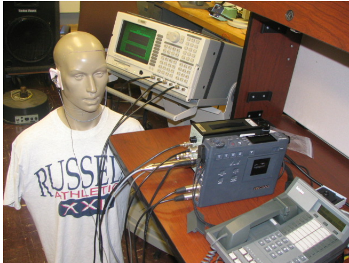
Figure 4 Test Setup of the Dictaphone C-Phone System Using KEMAR Kaiser-Permanente California HETA 2003-0273;-0280;-0287
