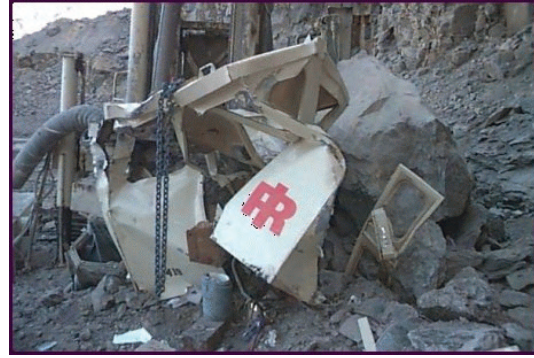
Figure 4. Cab crushed by slope failure (MSHA fatalgram, www.msha.gov).
