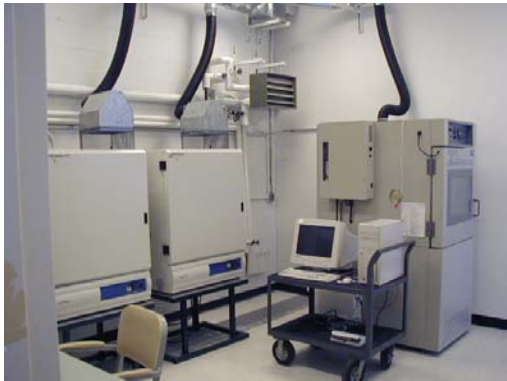
Figure 2 Convection ovens and environmental chamber for accelerating aging in the ECTF
