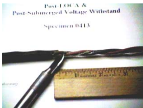
Typical cable specimen tested in the ECTF.
