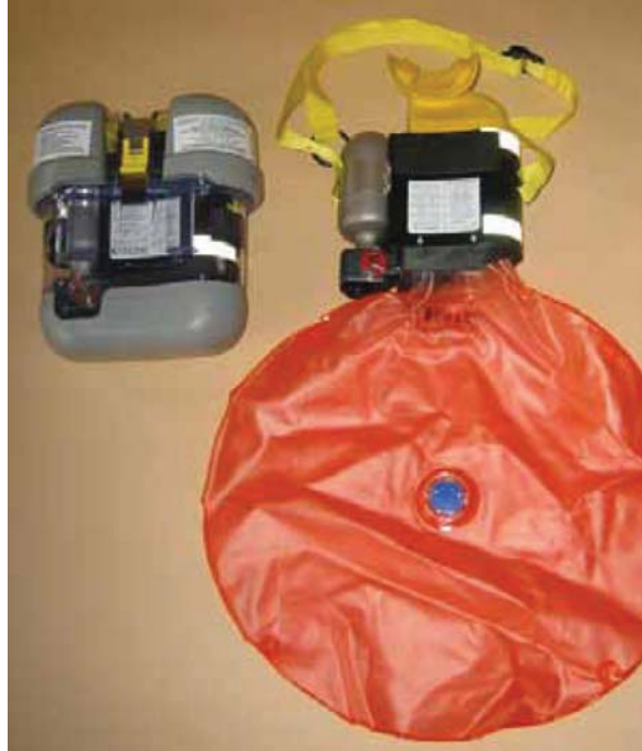
Figure 7. Partially Uncased and Uncased Ocenco M-20 Self-rescuer
