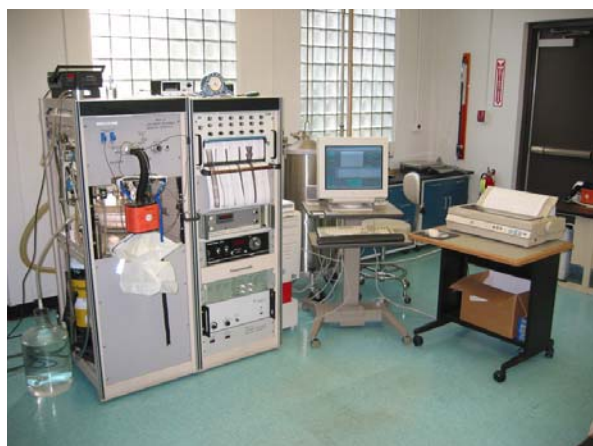
Figure 1. Breathing and Metabolic Simulator
