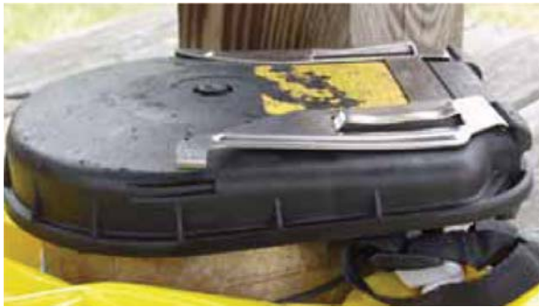
Figure 9. Dented Draeger OXY K-Plus Belt-Clip
