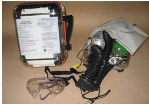
Figure 6. Cased and Uncased Ocenco EBA 6.5 Self-rescuer
