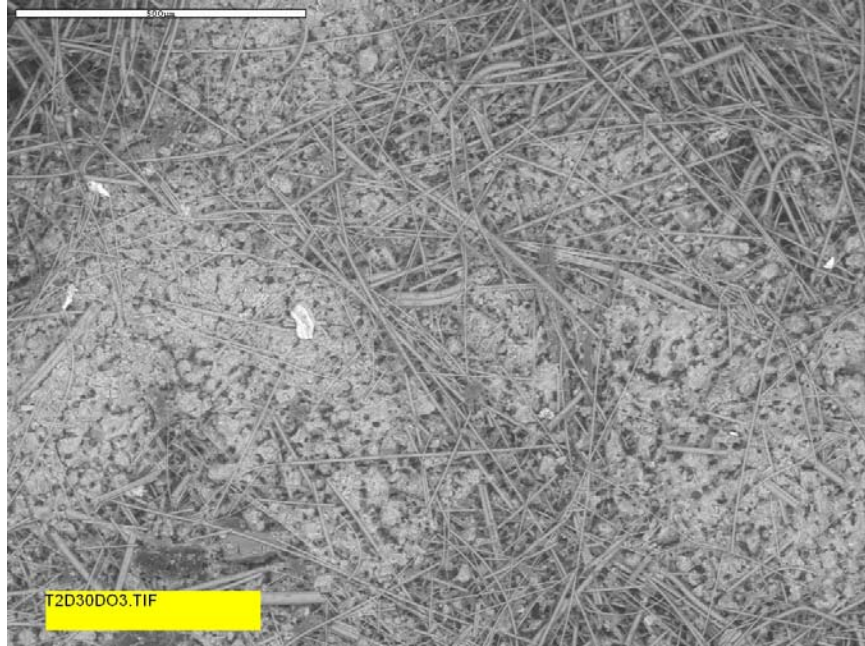
Figure D3-20. ESEM image for a Test #2, Day-30 exterior fiberglass sample on the drain collar. Image shows particulate deposits or growth on fiberglass. (T2D30DO3)
