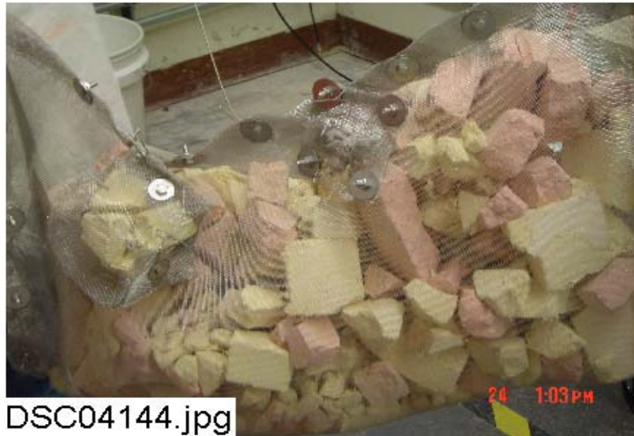
Figure 2-5. Solid pieces of cal-sil samples in SS mesh.
