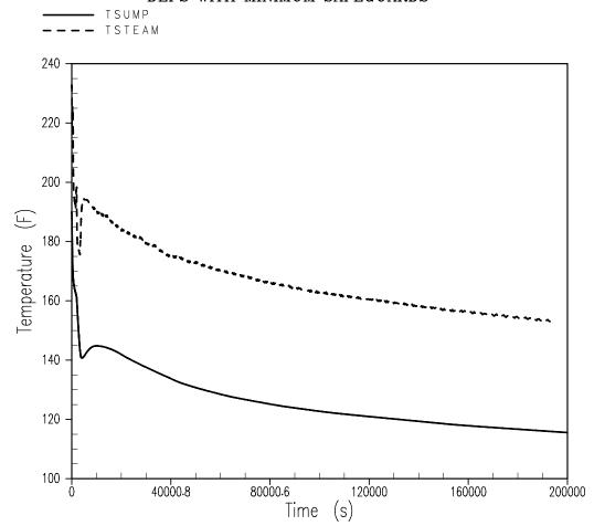
Figure 6: Four Loop Ice Condenser Plant Post-LOCA Temperature Profile (Linear Time Scale).
