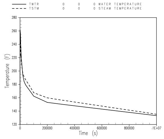
Figure 2: Four Loop Post-LOCA Temperature Profile (Linear Time Scale).
