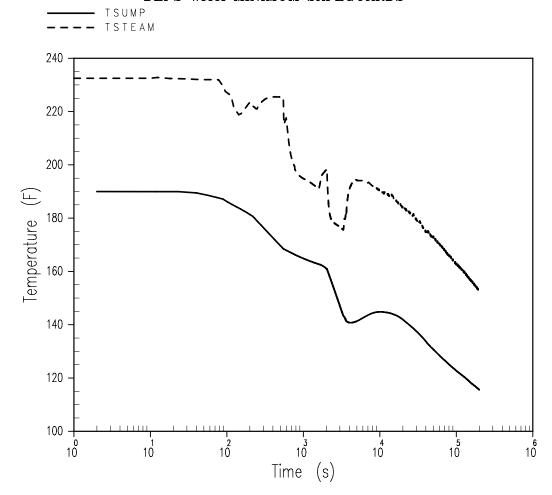
Figure 7: Four Loop Ice Condenser Plant Post-LOCA Temperature Profile (Logarithmic Time Scale).
