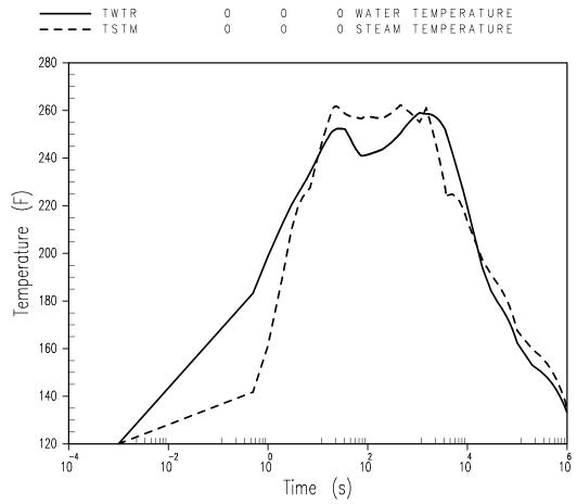
Figure 3: Four Loop Post-LOCA Temperature Profile (Logarithmic Time Scale).
