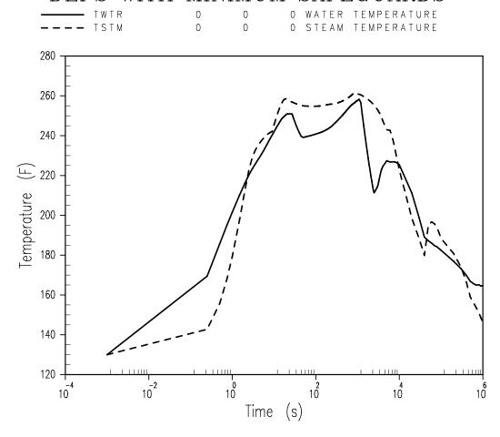
Figure 5: Three Loop Post-LOCA Temperature Profile (Logarithmic Time Scale).
