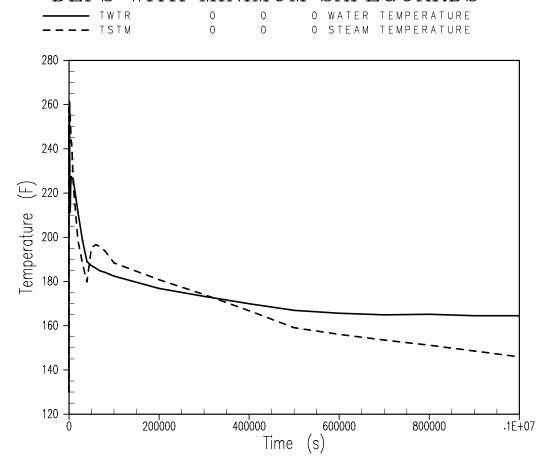
Figure 4: Three Loop Post-LOCA Temperature Profile (Linear Time Scale).
