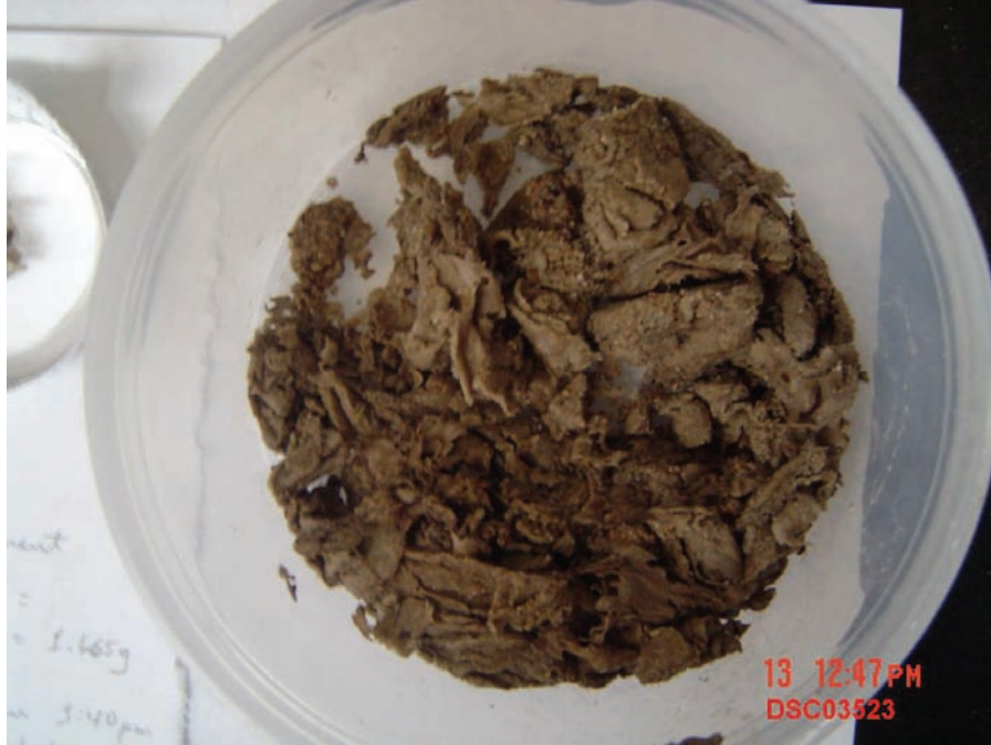
Figure 4-74. Sediment from south quadrant of tank after Test #1.
