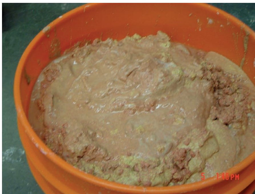
Figure 4-84. Sediment removed from the tank after Test #3.
