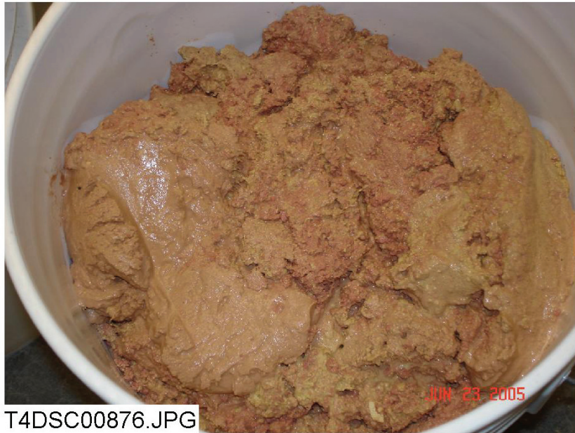
Figure 4-90. Sediment removed from the tank after Test #4.
