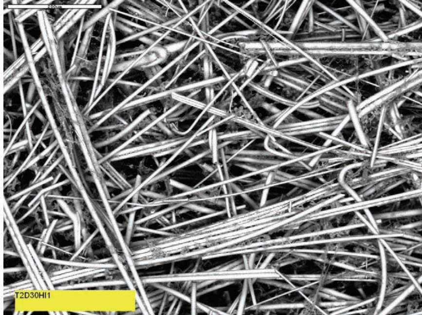
Figure 4-32. ESEM image for a Test #2, Day 30, high-flow interior fiberglass sample.
