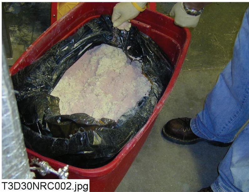
Figure 2-6. Pulverized cal-sil insulation before addition to the ICET tank.
