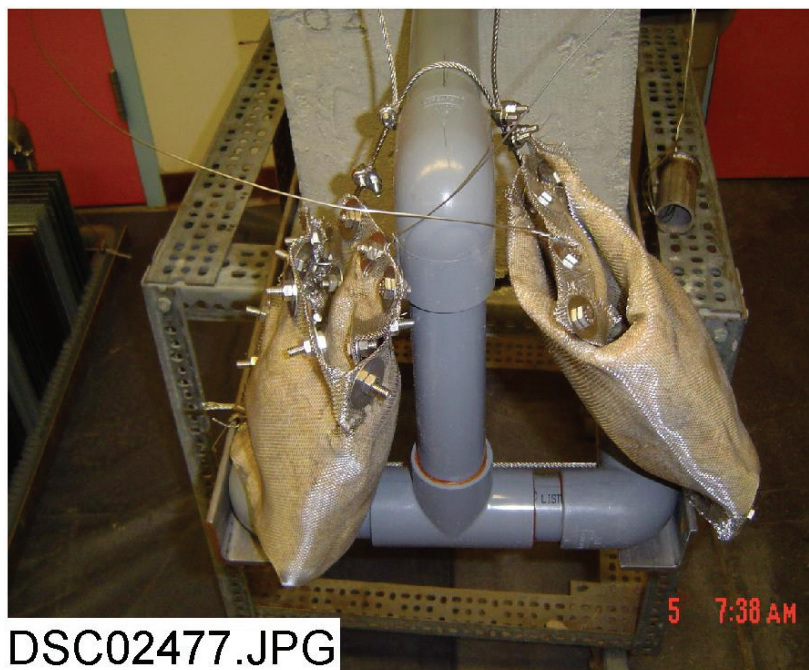
Figure 2-4. Fiberglass samples attached to a coupon rack.
