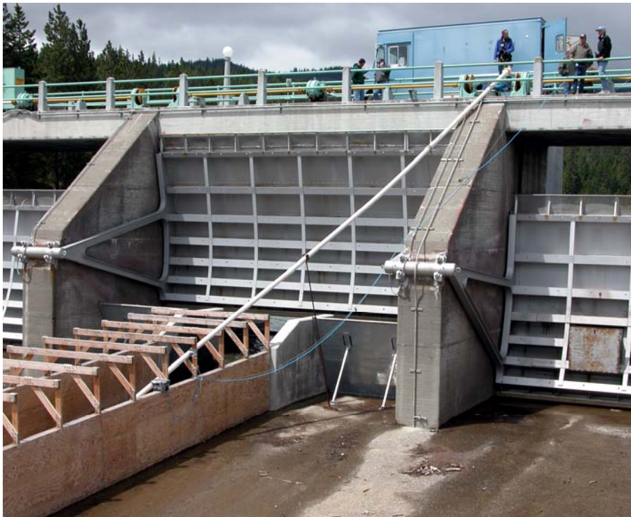
The release apparatus provided by the Bureau of Reclamation for the fish testing
