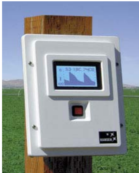
Figure 9 - Soil moisture data recorder with graphing
