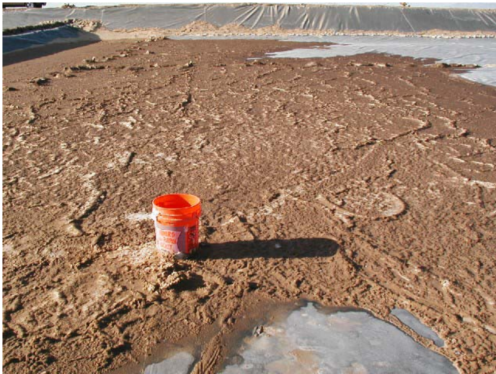
Figure 5.6—Bitterns after 2 weeks of evaporation at Salton Sea Test Base.
