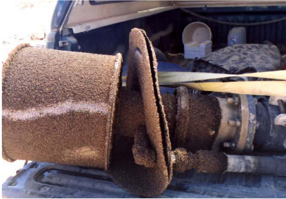
Figure 5.9—Barnacle fouling of Salton Sea Test Base fish screen.
