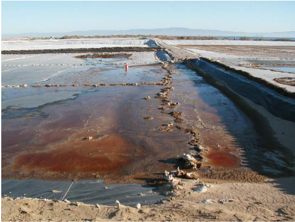
Figure 5.5—Bitterns during final evaporation at Salton Sea Test Base.
