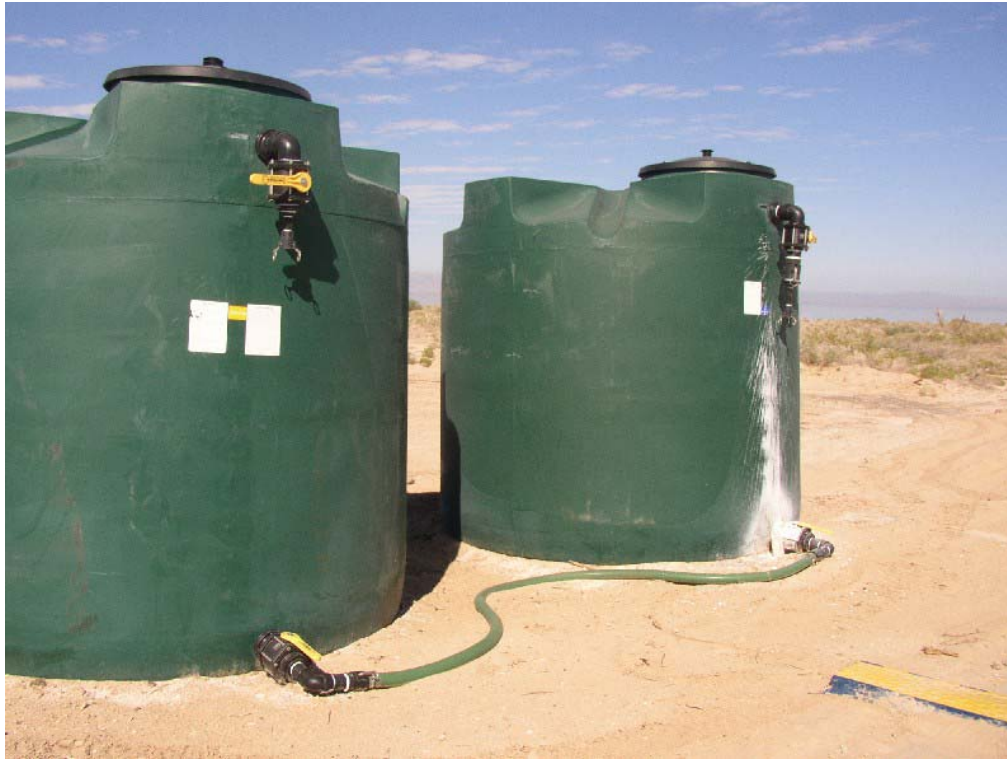
Figure 4.11—Supply tanks with heavy brine used in salt deposit density increase test (test 2).
