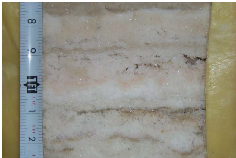
Figure 4.25—Salton Sea undisturbed salt block sample 54F-138, pad 6, excavation No. 13.
