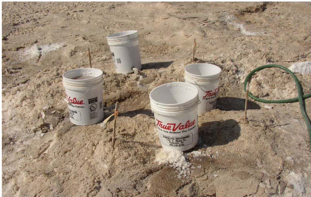
Figure 4.10—Heavy brine dripping onto deposits on core pad 7.
