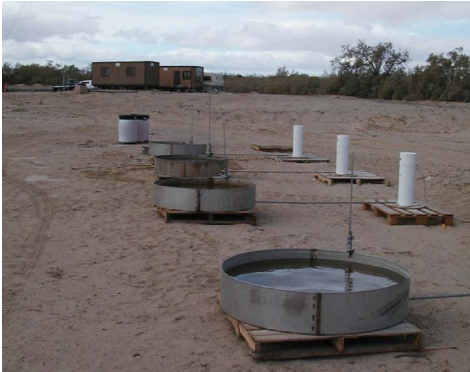
Figure 2.2—Class A pans for brine evaporation studies.
