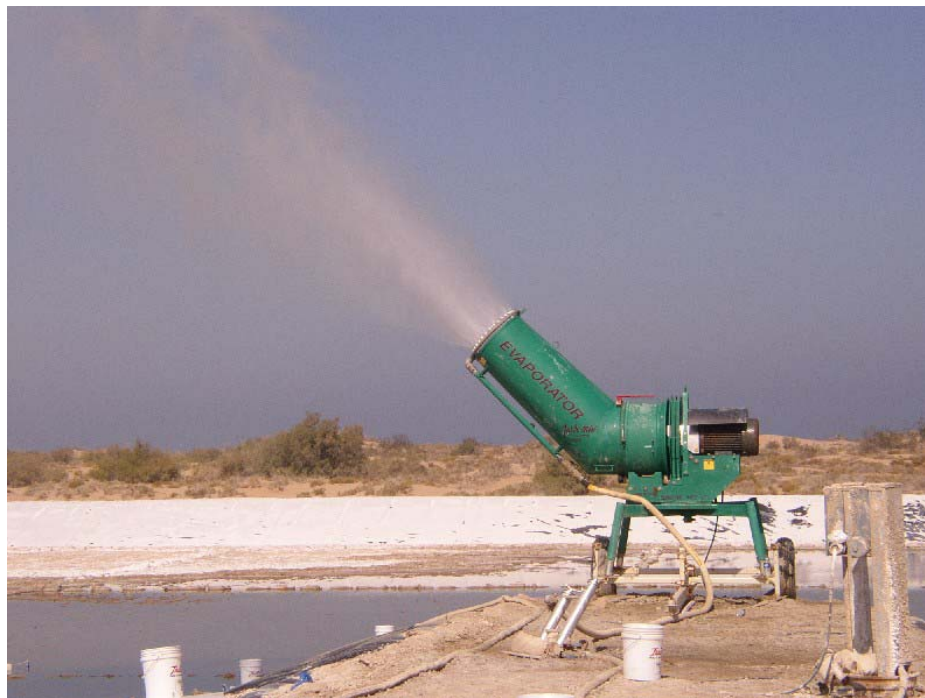
Figure 5.13—Slimline evaporator used in power use study.
