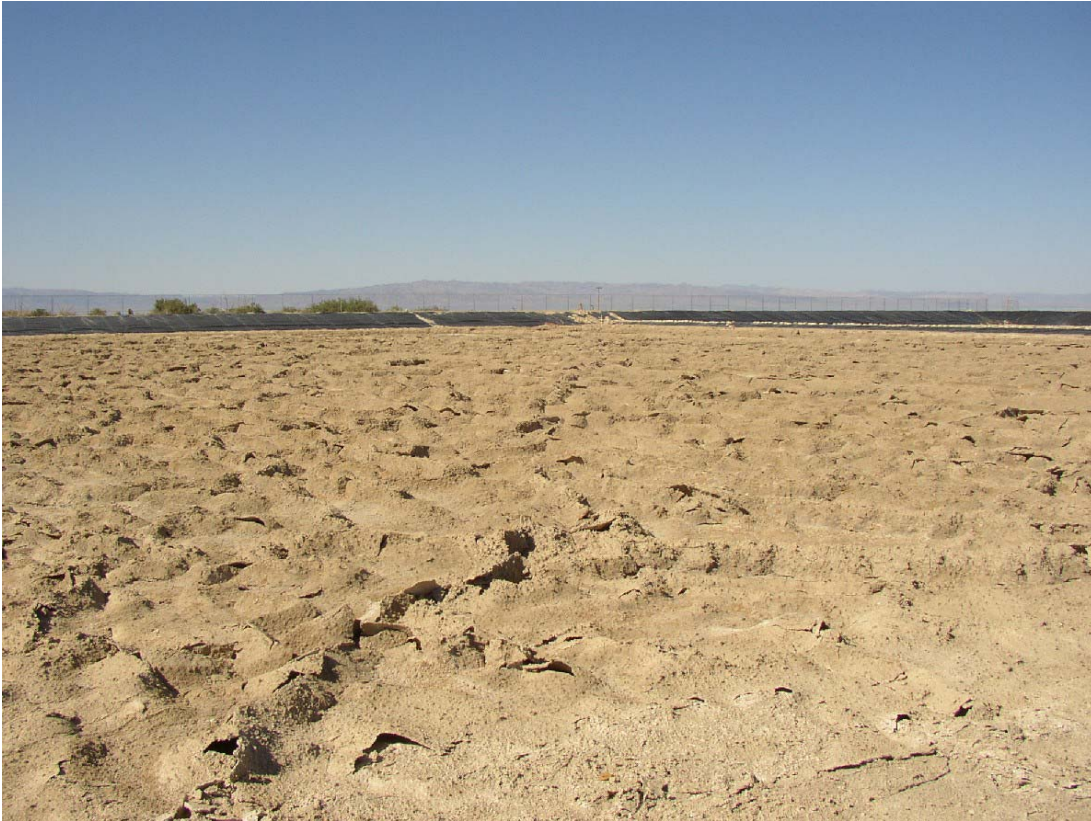
Figure 4.9—Salts reached dryness in disposal pond
