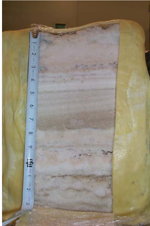
Figure 4.22—Salton Sea undisturbed salt block sample 54F-138, pad 6, excavation No. 13.
