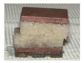
Appendix F16 – Direct Shear Test Photos of Specimen 3 (30 lb/in² Normal Stress) at 0.00003 in/min Strain Rate, 54F-136 (After Test)
