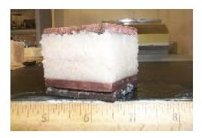
Appendix F8 – Direct Shear Test Photos of Specimen 4 (60 lb/in² Normal Stress), 54F-132 (After Test)
