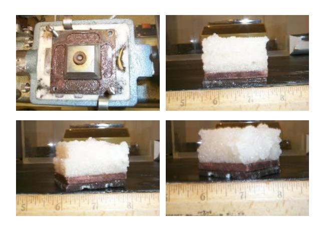
Appendix F13 – Direct Shear Test Photos of Specimen 1 (7.5 lb/in² Normal Stress), 54F-136 (After Test)
