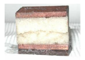
Appendix F19 – Direct Shear Test Photos of Specimen 2 (15 lb/in² Normal Stress), 54F-138 (After Test)
