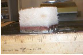
Appendix F11 – Direct Shear Test Photos of Specimen 3 (30 lb/in² Normal Stress), 54F-135 (After Test)
