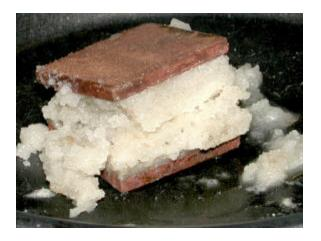
Appendix F17 – Direct Shear Test Photos of Specimen 4 (60 lb/in² Normal Stress), 54F-136 (After Test)
