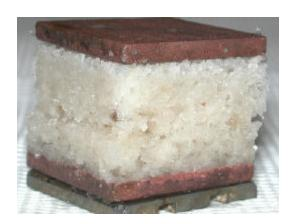
Appendix F15 – Direct Shear Test Photos of Specimen 3 (30 lb/in² Normal Stress), 54F-136 (After Test)
