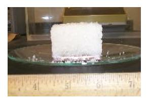
Appendix F3 – Direct Shear Test Photos of Specimen 3 (30 lb/in² Normal Stress), 54F-128 (After Test)
