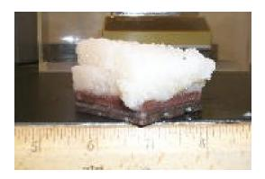
Appendix F2 – Direct Shear Test Photos of Specimen 2 (15 lb/in² Normal Stress), 54F-128 (After Test)
