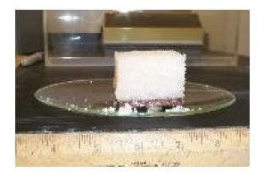
Appendix F5 – Direct Shear Test Photos of Specimen 1 (7.5 lb/in² Normal Stress), 54F-132 (After Test)
