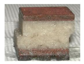
Appendix F18 – Direct Shear Test Photos of Specimen 1 (7.5 lb/in² Normal Stress), 54F-138 (After Test)
