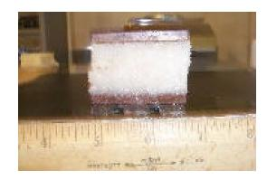
Appendix F7 – Direct Shear Test Photos of Specimen 3 (30 lb/in² Normal Stress), 54F-132 (After Test)
