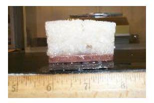
Appendix F12 – Direct Shear Test Photos of Specimen 4 (60 lb/in² Normal Stress), 54F-135 (After Test)
