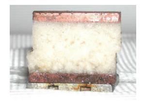
Appendix F21 – Direct Shear Test Photos of Specimen 4 (60 lb/in² Normal Stress), 54F-138 (After Test)
