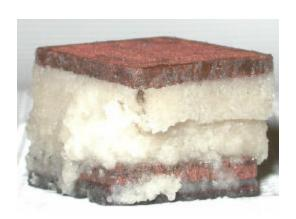
Appendix F20 – Direct Shear Test Photos of Specimen 3 (30 lb/in² Normal Stress), 54F-138 (After Test)
