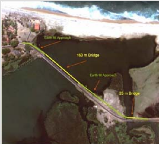
An aerial view of Arugam Bay showing design of the new bridge under construction by USAID.
