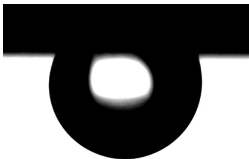
Fig. 18 - A decane drop surrounded by water on a mica sample treated with Crude A
