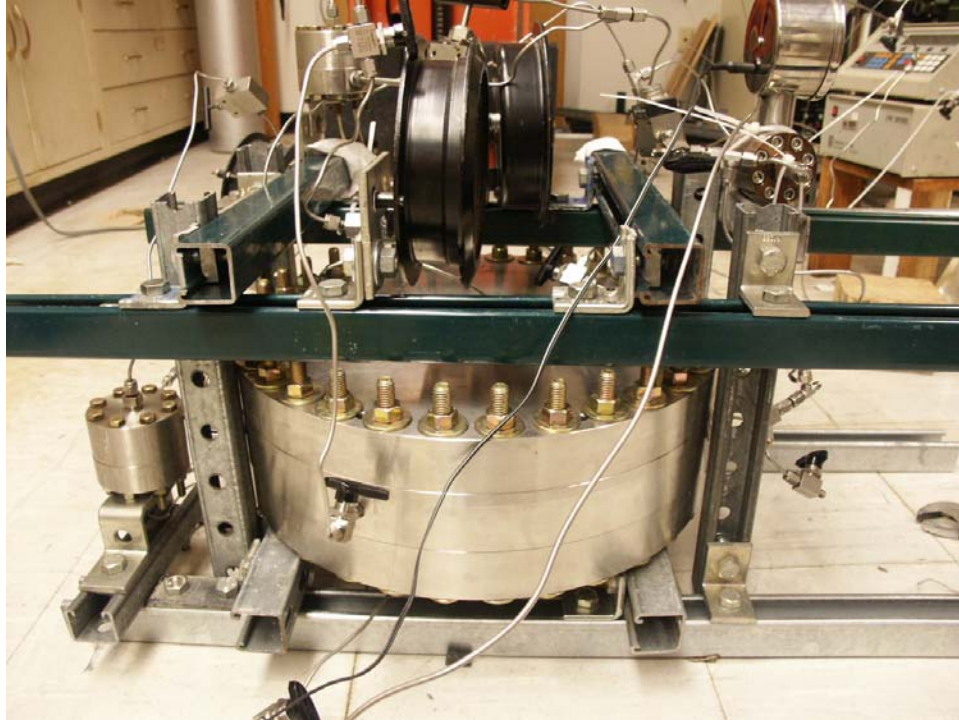
Fig. 5 - Side view of the 5-spot high-pressure cell
