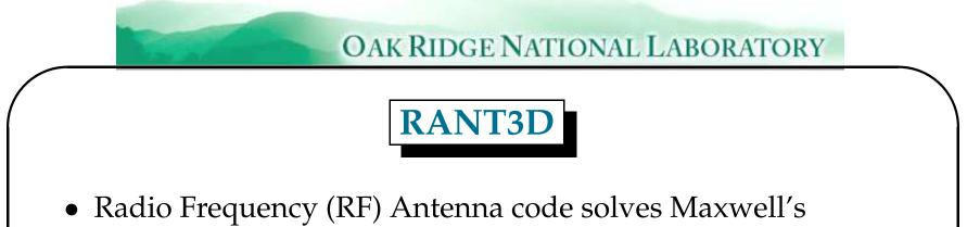
• Radio Frequency (RF) Antenna code solves Maxwell's equations in Cartesian geometry using spectral basis is used in the design of antenna for heating and current drive in tokamaks. Each cavity uses variable separable representation.
