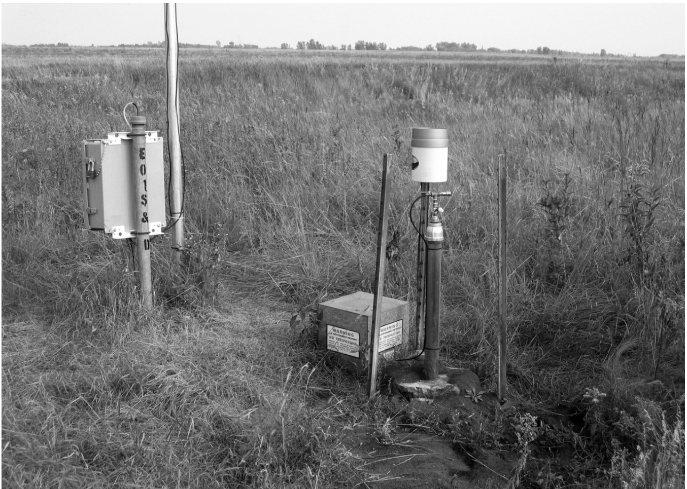
Ground-water observation well at Glacial Ridge, 2003
