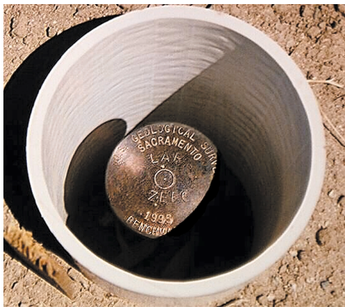
This bench mark was established in 1995 to monitor potential land subsidence in the Antelope Valley, Mojave Desert, California.
