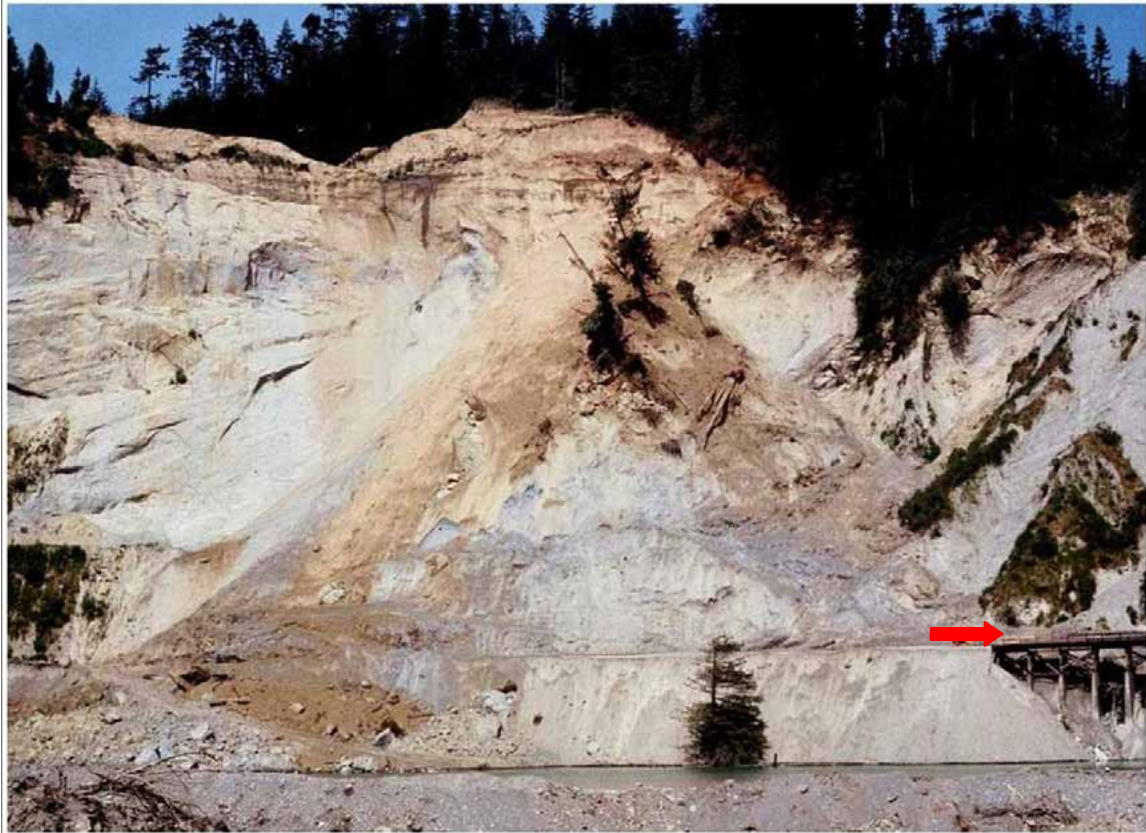
Figure 3-32. Photo of a Category 1 rock fall along the Scotia Bluffs adjacent to the Eel River near Fortuna, California. The triggering earthquake was the Fortuna, California, 7 June 1975, M_l 5.2 event. Note the disaggregated nature of the failed material, the steep slope, and the orange tractor (at red arrow) for scale. (Photograph by David Keefer, USGS, 1975.)
