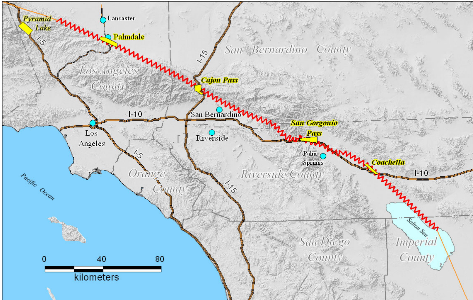
Figure 4-1. Principal lifeline corridor focus areas. Red line enotes rupture of southern San Andreas Fault in the ShakeOut Scenario.
