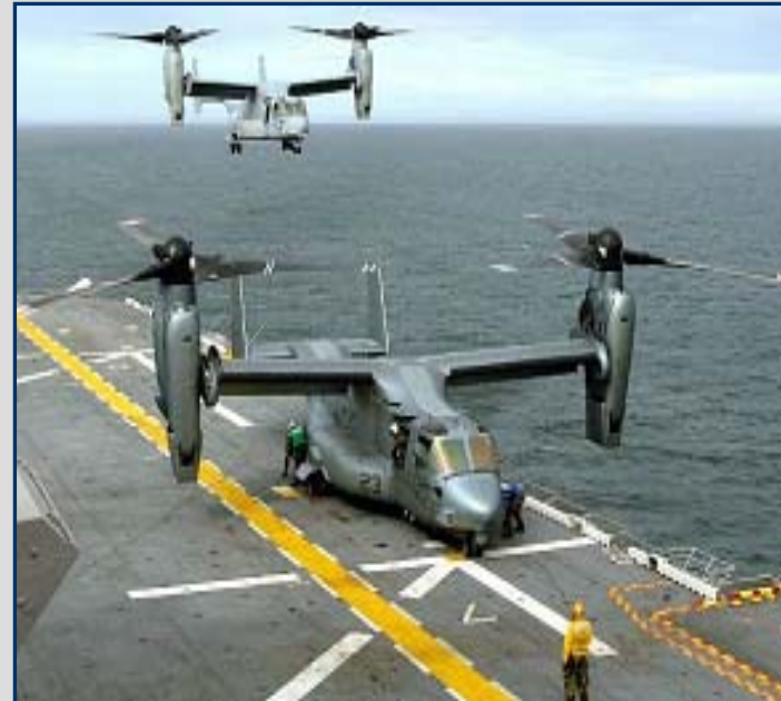
A Marine Corps MV-22B Osprey prepares to refuel while another Osprey approaches the flight deck of the amphibious assault ship USS Wasp (LHD 1) for landing.
