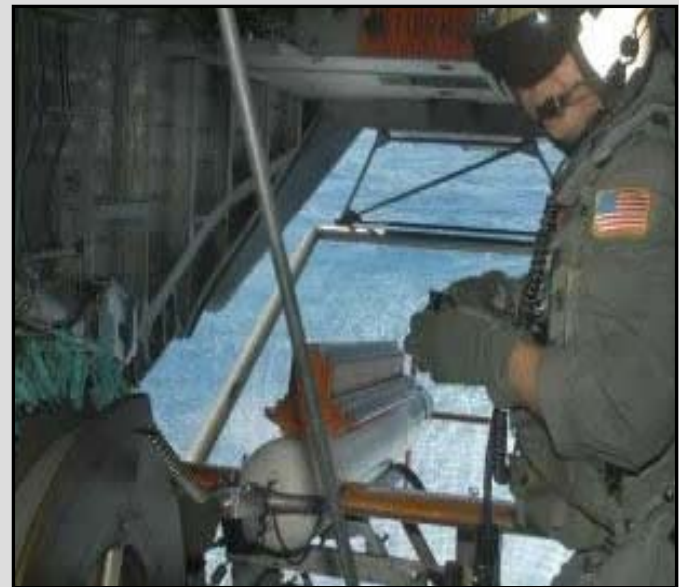
Aviation Electrician's mate 2nd Class maneuvers an AQS-24 mine locator, which is designed to use sonar and laser technology to photograph underwater mines.
