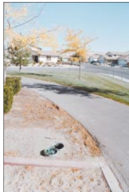
Shallow monitoring well in Reno-Sparks urban area, October 1995. Photograph by Michael S. Lico, U.S. Geological Survey.
