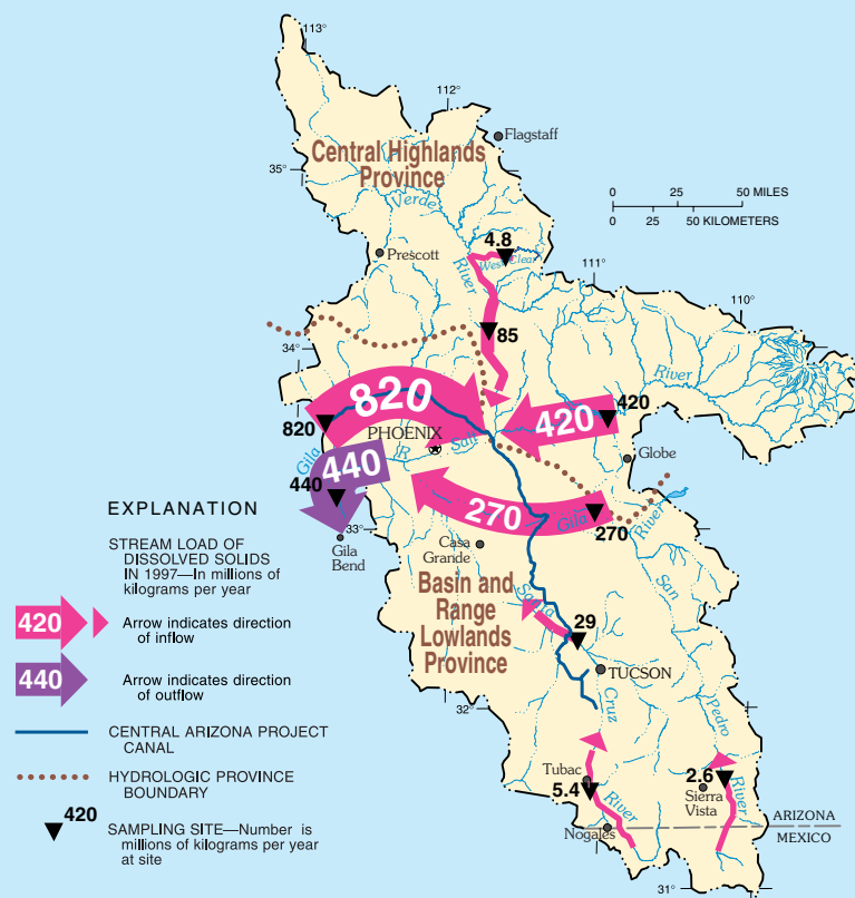
Figure 8. Streams and the CAP canal brought 1.6 billion kilograms of dissolved solids into the Basin and Range Lowlands in 1997, but only 440 million kilograms left the area in streams. The remaining dissolved solids accumulated in soils, the unsaturated zone, and ground water.
