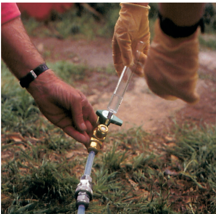
Figure 19. Samples are collected at the well head for radon analysis to prevent possible sample contamination from exposure to the atmosphere.
