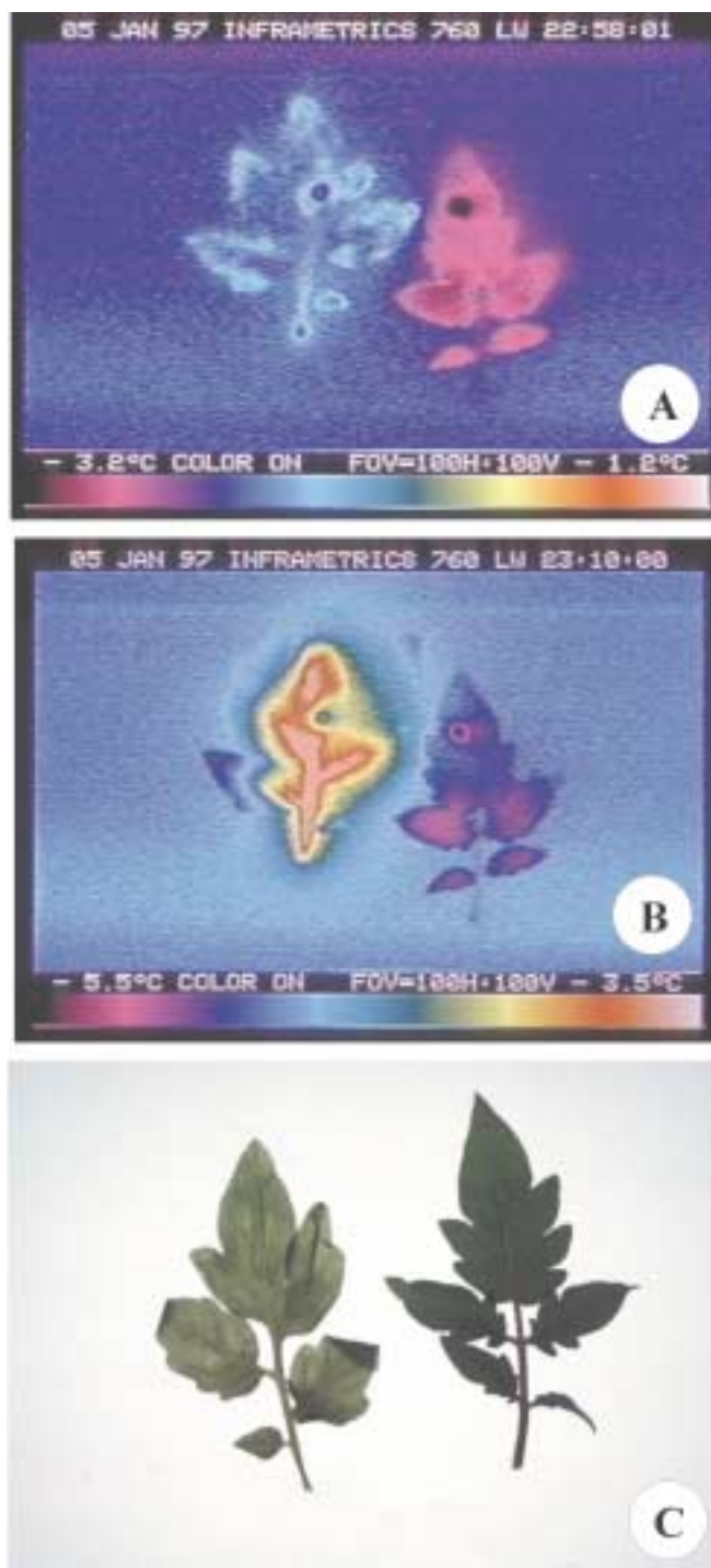
Fig. 2. Exposure of noncoated and M96-018-coated tomato leaflets to freezing temperatures. A droplet of water containing Ice + bacteria was placed on the upper surface of each leaf. (A and B) Infrared images; (C) a photograph of the leaves after they were returned to room temperature and the hydrophobic particle film was removed. The droplet of Ice + bacteria froze at about -1.5 °C on both leaves. The frozen droplet induced the noncoated leaf to freeze (A, left) while the coated leaf remained nonfrozen (A, right). The coated leaf was still nonfrozen at -5.5 °C (B, right). After removal from the environmental chamber and warming (C), the noncoated leaf appeared completely water soaked (left) while the M96-018-treated leaf (right) appeared completely turgid and noninjured.
