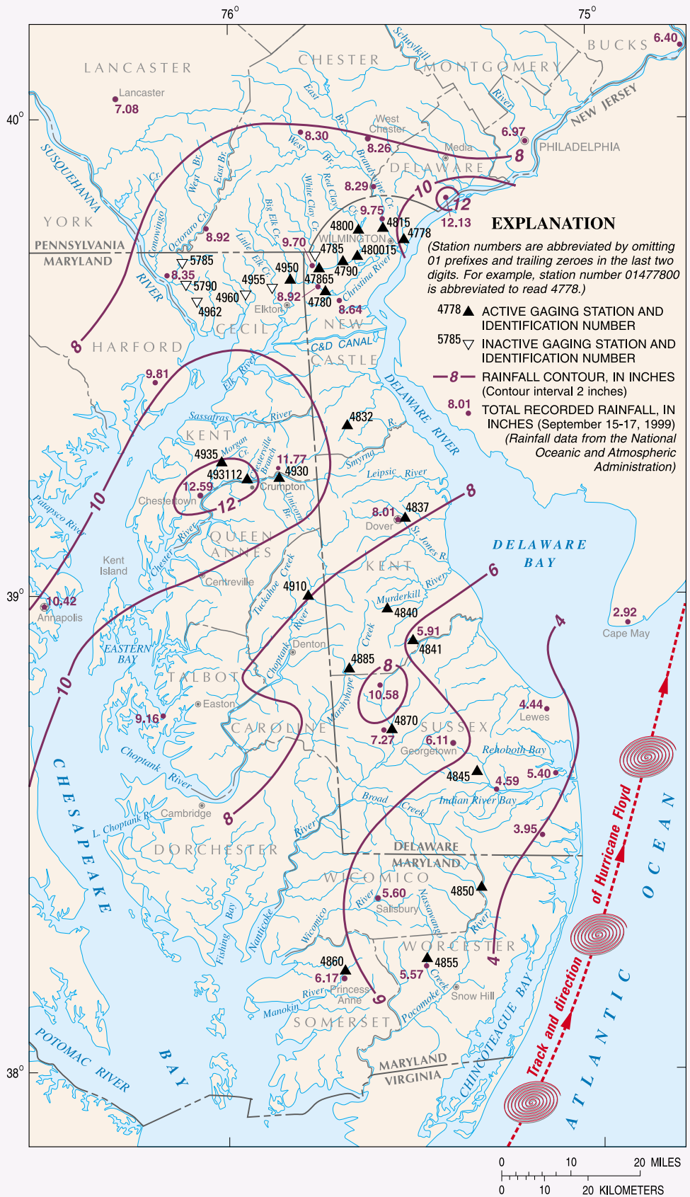
Figure 1. Location of active and inactive streamflow-gaging stations in Delaware and the Eastern Shore of Maryland, rainfall distribution, and track and direction of Hurricane Floyd, 1999.
