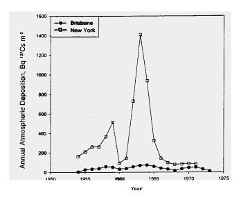
I Figure 1 The history of bomb fallout  $_{\rm 37CS}$  deposition (as calculated from  $_{\rm 90Sr}$  measurements) in New York city, NY, USA and Brisbane, Queensland. Australia. The data are from the Environmental Measurements Laboratory website
