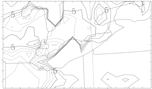
FIG. 1. Mean surface roughness length (meters) used in the standard roughness case. Fractional parts of each grid cell can have different land cover types and hence different surface roughness lengths. Contours are shown for values from 0.1 to 0.7 m, with dashed contours for values below 0.5 m. No land areas have surface roughness lengths greater than 0.8 m. Grid cells that are completely covered by water are assigned a default roughness length of 2.0 m that is used for purposes of this figure, but see the text for the treatment of roughness length over water.
