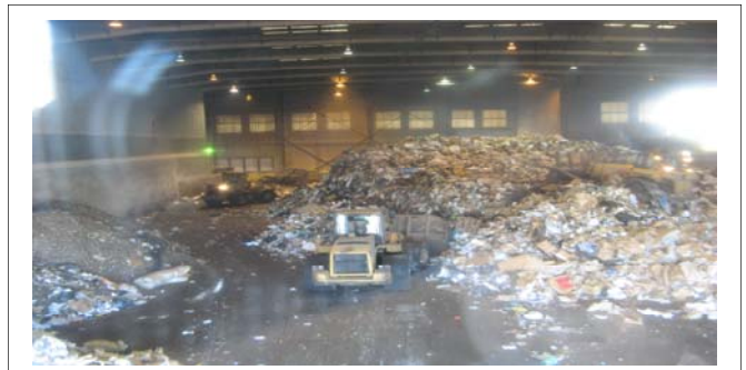
Trash processed at H-Power is incinerated, which then fuels steam turbines that generate electricity. The facility processes about 2,000 tons of waste a day and generates enough power for about 45,000 homes.
