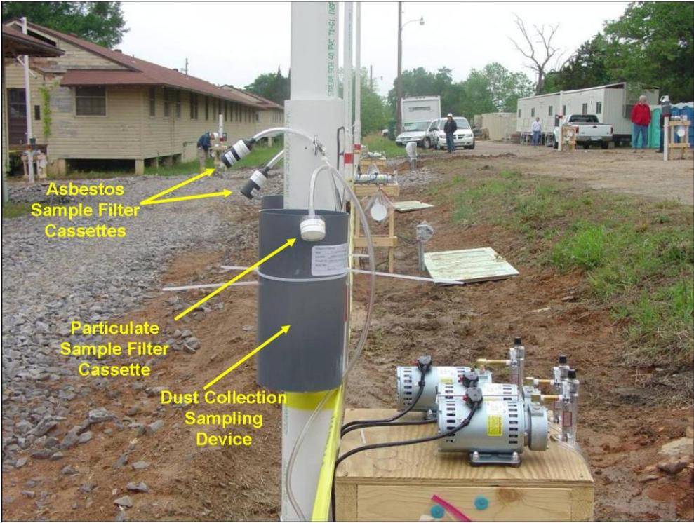
Figure 4-13. The five-ft high sampling array on the inner ring (Ring One).
