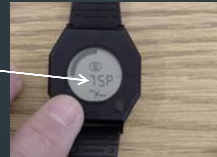
Button press to view “ Performance-Readiness, ” which is displayed as a percentage (P) from 0-99%; in this example, as “75P” or 75% optimal.
